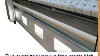
Two oversized vacuum fans create high power suction in the chute for best shake out performance. High speed throw-in rollers are throwing the items into the chute. The spreader brushes contribute to the spreading performance.
